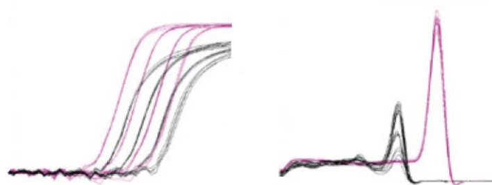
Visible blue samples, earlier Ct values, superb sensitivity achieved with ORA™ SEE qPCR Green Mixes. Amplification & melt traces of mouse actin gamma-1 housekeeping gene from a cDNA dilution series; ORA™ SEE qPCR Green Mix (purple) and Competitor Mix (black).
